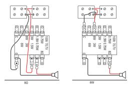
Circuit diagrams 8 Ohm and 6 W connection
